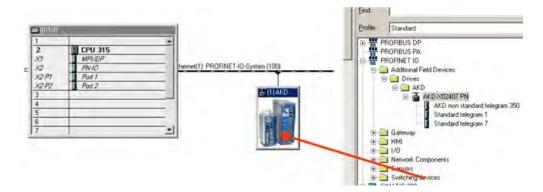
7. Now configure the telegram, for example telegram 7 for use in position mode. Drag and drop telegram 7 into slot 1.
