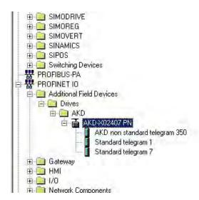
6. Click on the AKD device (not a telegram) and connect it to the PLC (drag and drop)
