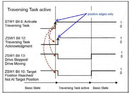
If another motion task shall be executed before the current motion task has finished ("Change on the fly"), the "Activate traversing task" Bit in STW1 can be directly cleared (after the setting of Bit 12 in ZSW1 was detected). In addition, the drive will clear Bit 12 in ZSW1. After this another motion task can be loaded. If an error occurs or the configured motion task can not be executed, bit 12 in ZSW1 will not be set.
