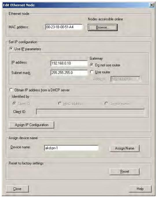
You will usually see a status message that indicates that the change was successful and the AKD display will show the new address. If you receive a failure message, make sure that no IO connection is currently running, then retry the address or name change.
