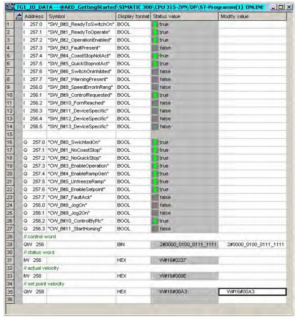
Now the set point velocity can be set. In the example (see variable table) the value is QW 258 is 0xA3 (60 rpm ("Units" (=> p. 40))). To start the motion, set Bit 4, 5 and 6 (enable ramp generator, unfreeze ramp generator and enable new set point).
