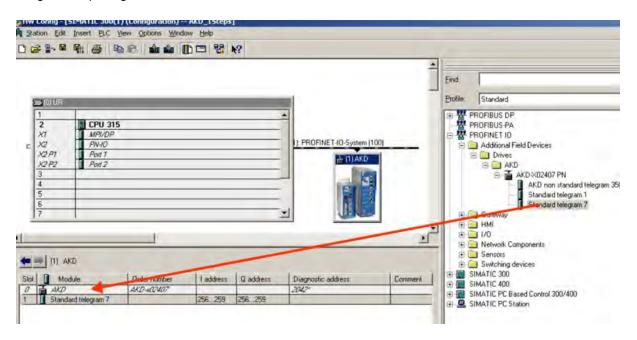
8. Double click on the PROFINET network (line which connects PLC and AKD) and configure the update time. Click OK for closing this window.
