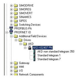
6. Click on the AKD device (not a telegram) and connect it to the PLC (drag and drop)
