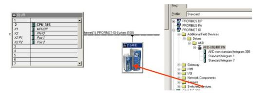
7. Now configure the telegram, for example telegram 7 for use in position mode. Drag and drop telegram 7 into slot 1.
