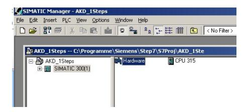
3. Go to Options and click "Install GSD Files". Here also the GSDML files for PROFINET devices can be installed.:
