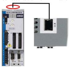
Connect the service interface (X11) of the drive to an Ethernet interface on the PROFINET Master directly or via a network switch, while the supply to the equipment is switched off.
