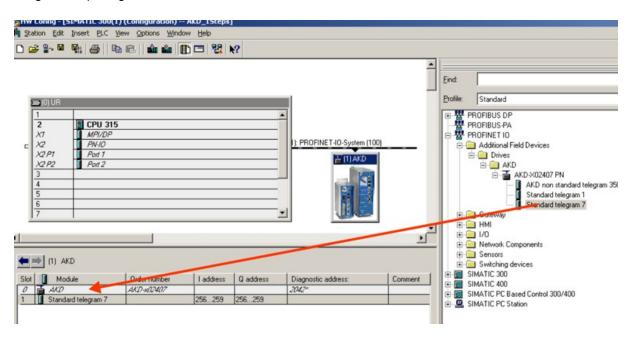
8. Double click on the PROFINET network (line which connects PLC and AKD) and configure the update time. Click OK for closing this window.
