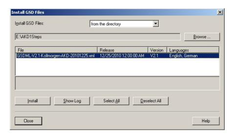
5. The AKD GSDML file is installed now and can be found in the SIMATIC hardware catalog. Open PROFINET I/O->Additional Fieldbus Devices->Drives->AKD
