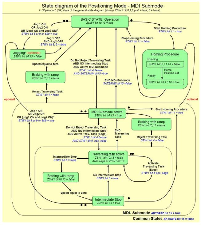
The activation of a new motion task (or traversing task), is done through a hand shake algorithm. After setting the "Activate traversing task" bit 6 in STW1, the signals MDI\_TARPOS, MDI\_VELOCITY, MDI\_ACC, MDI\_DEC and MDI\_MOD with their current values are loaded into the drive. The "Traversing Task Acknowledgment" bit 12 in ZSW1 indicates the point in time, when the motion task is starting execution. The figure shows the behavior:
