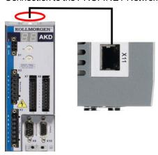
Connect the service interface (X11) of the drive to an Ethernet interface on the PROFINET Master directly or via a network switch, **while the supply to the equipment is switched off.**
