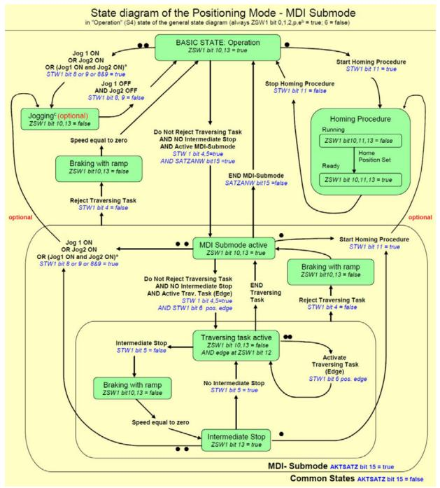
The activation of a new motion task (or traversing task), is done through a hand shake algorithm. After setting the "Activate traversing task" bit 6 in STW1, the signals MDI\_TARPOS, MDI\_VELOCITY, MDI\_ACC, MDI\_DEC and MDI\_MOD with their current values are loaded into the drive. The "Traversing Task Acknowledgment" bit 12 in ZSW1 indicates the point in time, when the motion task is starting execution.
