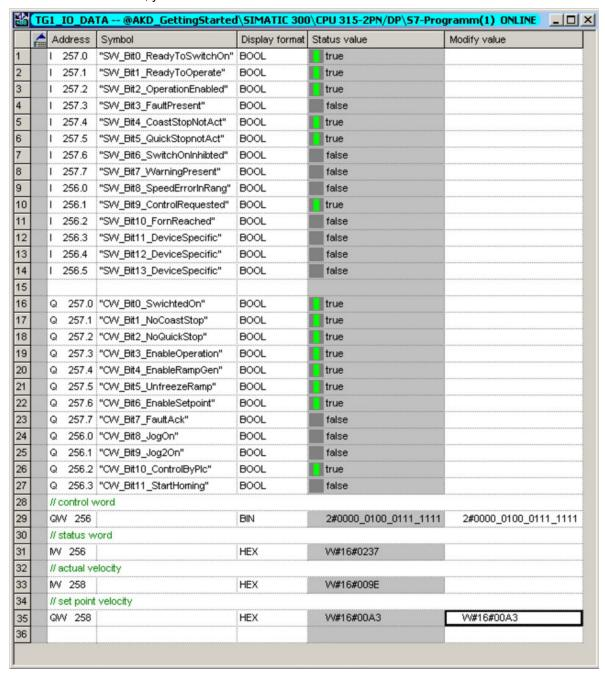
Now the set point velocity can be set. In the example (see variable table) the value is QW 258 is 0xA3 (60 rpm ("Units" (→ p. 42))). To start the motion, set Bit 4, 5 and 6 (enable ramp generator, unfreeze ramp generator and enable new set point).
