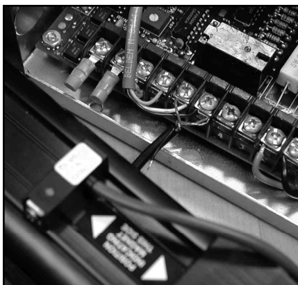
Limit switch sensors mounted to cylinder and wired to control
