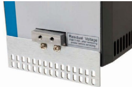
AKD-x02406 & xzzz07 types: flat grounding plate
