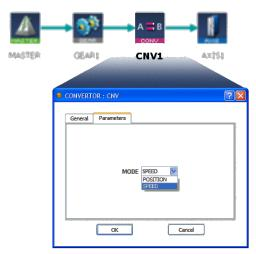
Change the mode of Converter block to SPEED (and not POSITION mode).
