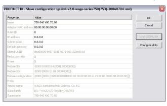
4. Do the slot configuration after the GSDML file import.
