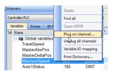
Figure 8-29: Plugging a Probe from the Dictionary
