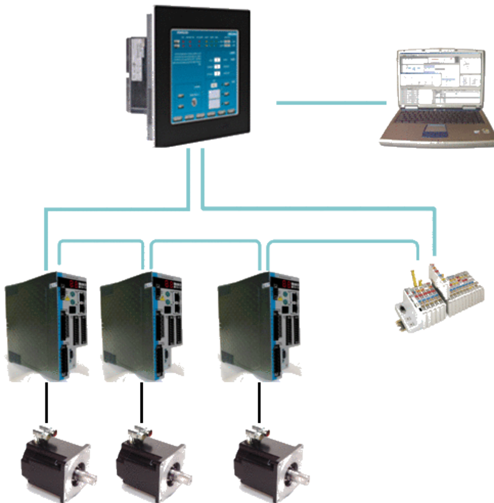
Figure 2-6: Example of Automation System
