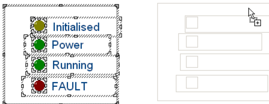
Figure 7-34: Control Panel - Selection of Controls
