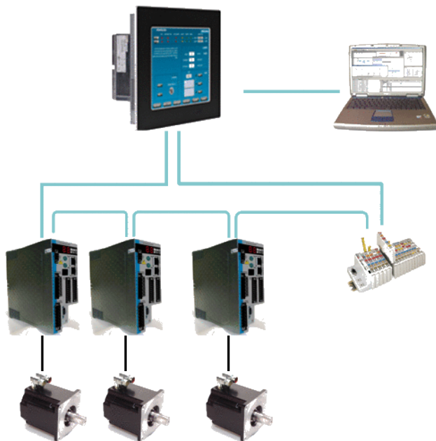
Figure 2-6: Example of Automation System
