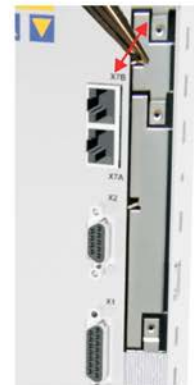
6 - Pull out the top plate
