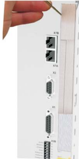
2 - Detach the film (at the perforations)
